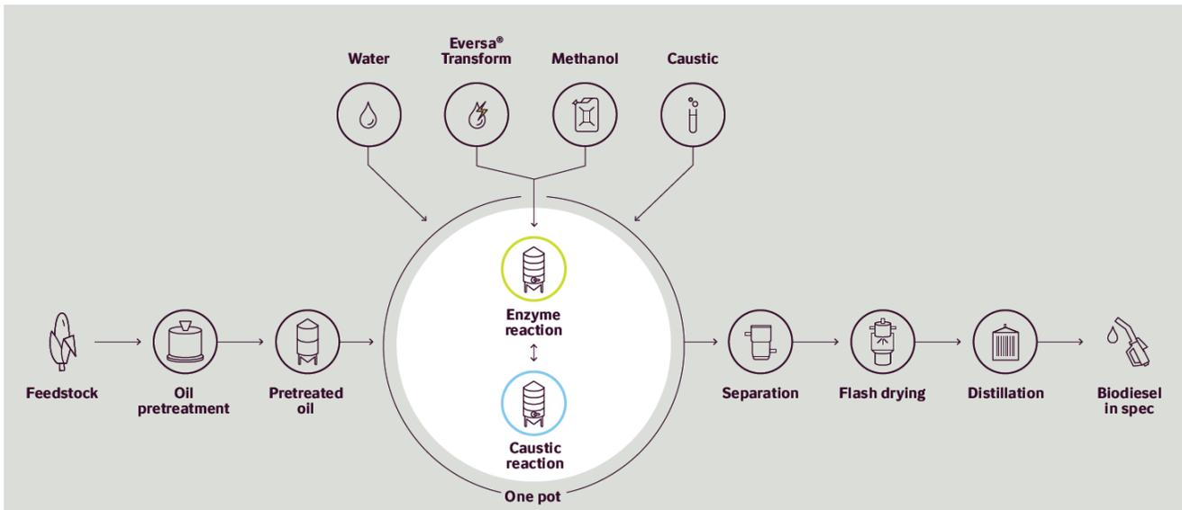
Fig. 1. The basic layout of the enzymatic process. Recommended conditions for the enzyme reactor: 0.3–0.4% Novozymes Eversa® Transform 2.0 enzyme, 1.2–1.5 equivalent MeOH, 40°C/104°F, 1.5–2% water and 36 to 48 hours reaction time
